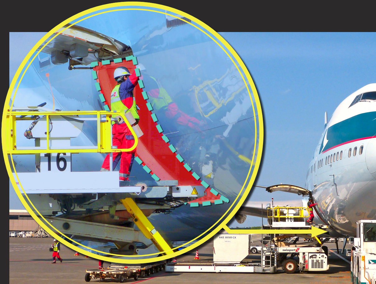
K-loader impact points can be protected with SENTIR bumpers and scissor lift crushing area with SENTIR contact edges
