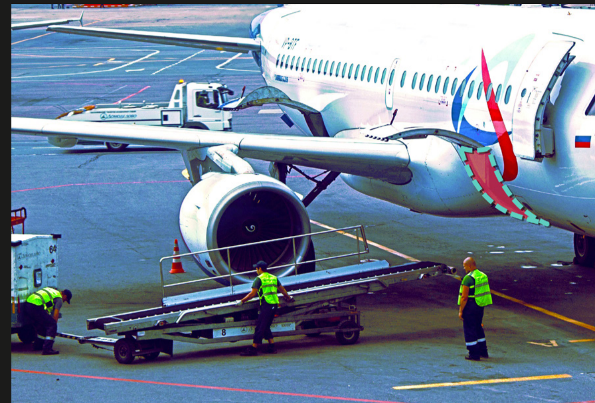
Belt Loaders for luggage can be fitted with SENTIR bumpers to protect aircraft to protect the hull
