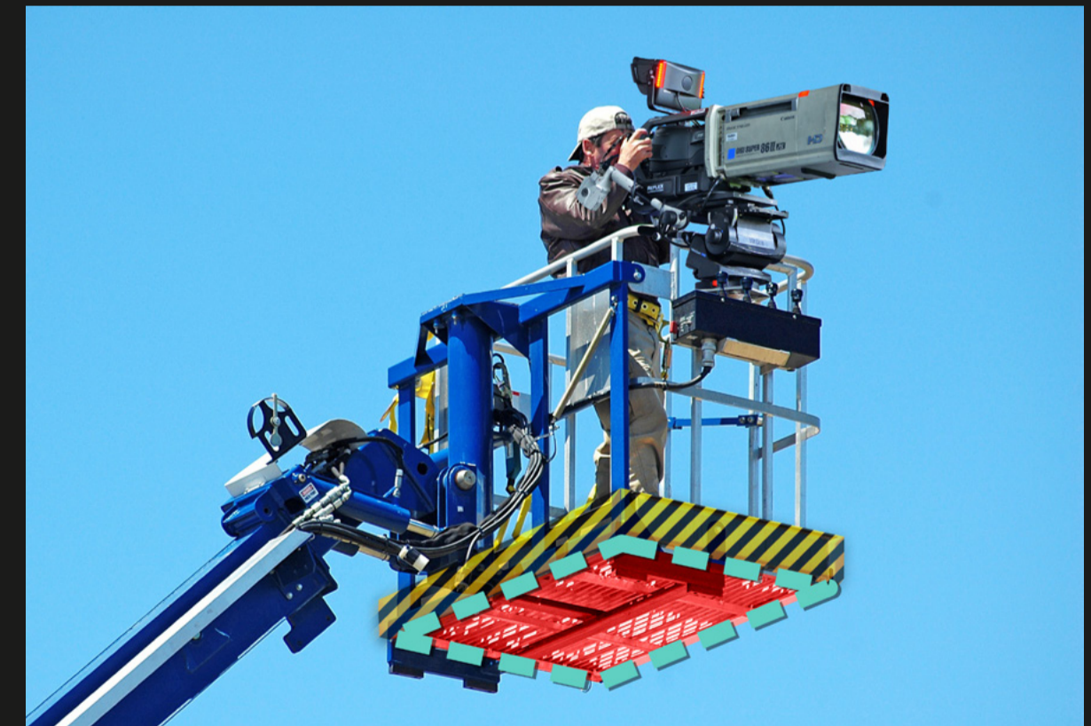
Aerial work platforms using SENTIR mats and bumpers to ensure worker safety against crushing and impact hazards
