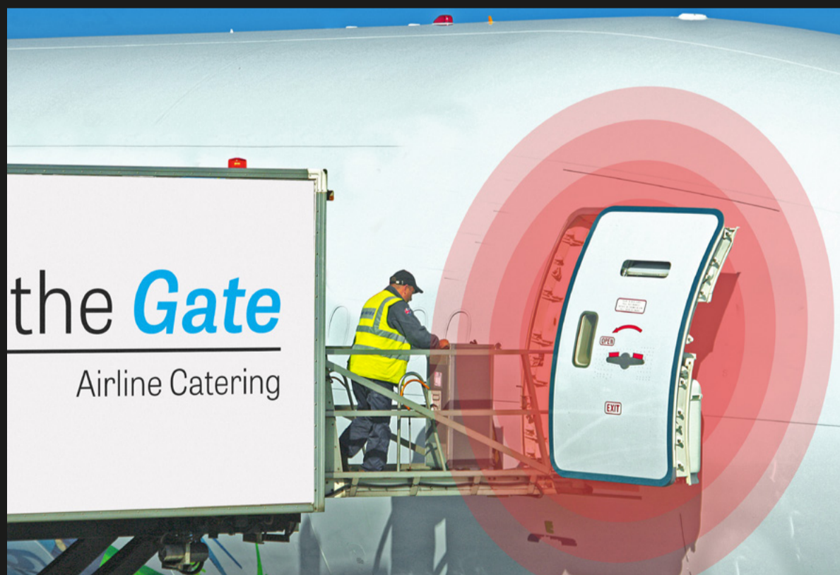
Catering truck impact points can be protected with SENTIR bumpers and scissor lift crushing area with SENTIR contact edges
