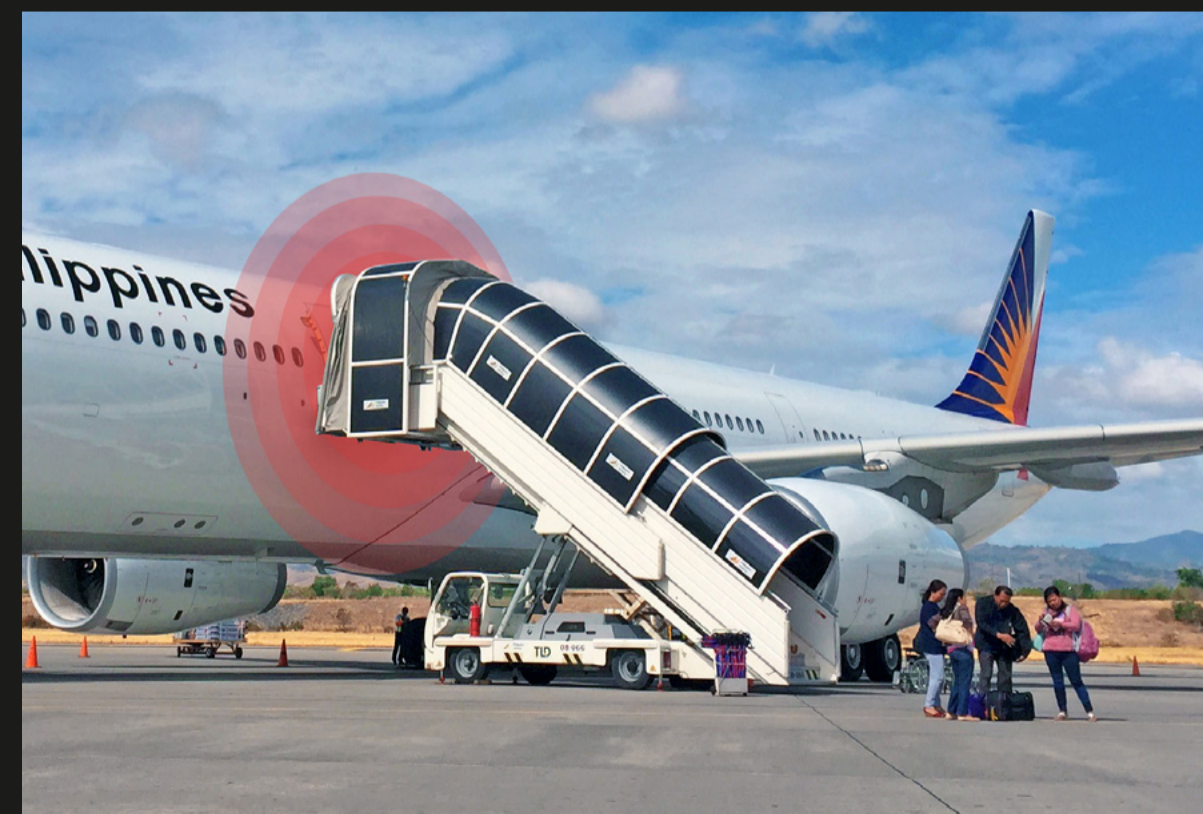
Mobile gangways fitted with SENTIR bumpers protect the aircraft from impact damage
