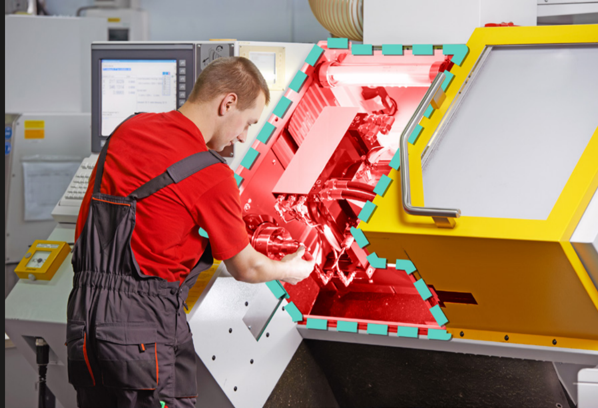
Operators can be protected from machine centre door crushing and shearing hazards with SENTIR contact edges , or machine functions disabled / slowed when in contact with a SENTIR mat
